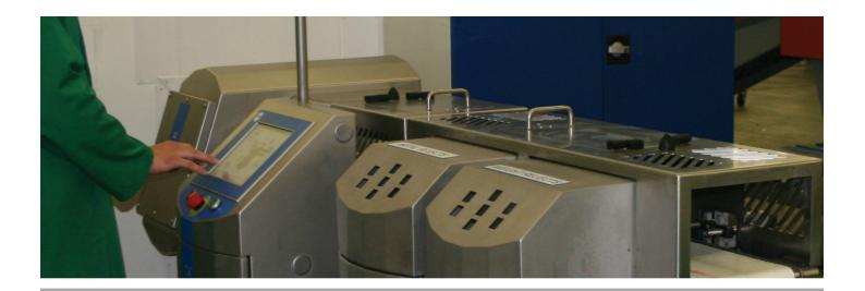
The Loma CW3 checkweigher design minimises vibration and enhances accuracy. Whatever your requirements, we have a model to suit. By networking these devices, we have succeeded in placing the checkweigher at the centre of the production environment, making it a source of information, which can help improve your company's bottom line. The CW3 will easily withstand real-world production line conditions and the intensive cleaning processes needed to maintain hygiene standards.
