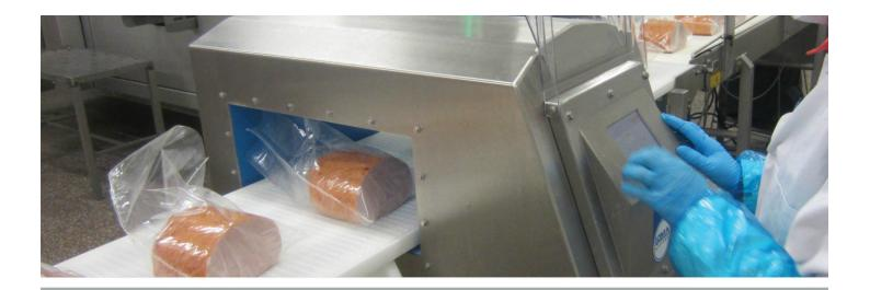
The launch of the Loma IQ3 Metal Detector was heralded as a revolution in metal detection technology due to its unique variable frequency operation, which means the unit can auto-select the correct frequency for maximum contaminant sensitivity. No longer are operators required
